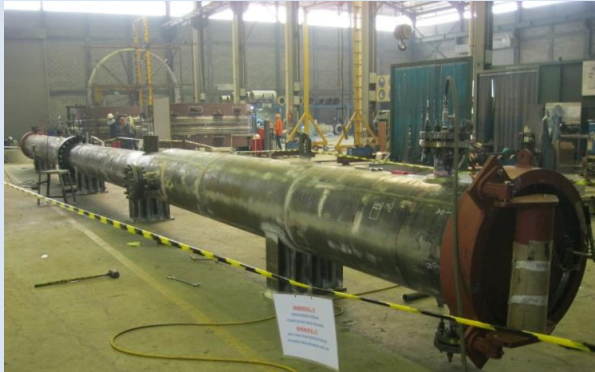
800 NB PIG LAUNCHER AND RECEIVER BEING HYDRO TESTED. THIS WAS SPECIALLY DESIGNED TO ACCOMMODATE EXTRA LONG INTELLIGENT PIGS.
