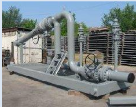
SPHERE PIG LAUNCHER WITH PIG PINS AND SPHERE PIG RECEIVER
