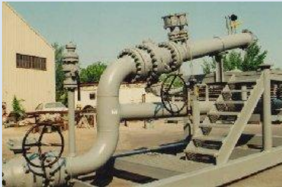
SPHERE PIG LAUNCHER WITH PIG PINS AND SPHERE PIG RECEIVER
